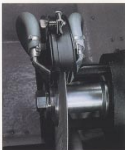
Twin hose jets apply coolant to both wheel and sample during cutting operation.
